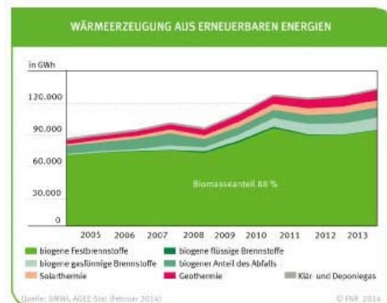
Figure 2: Heat generation from renewable energy sources
