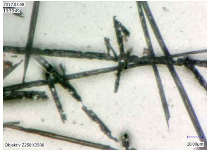
Optical microscopy image of a thermal treated CF sample (image: KIT).
