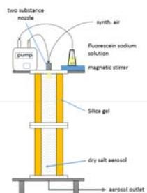
Standard aerosol generation according to the VDI guideline 3491
