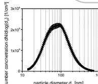
Number size distribution (left) and mass size distribution (right) of fluorescein sodium aerosol measured with a SMPS (DMA 3071, CPC 3775, TSI Inc., St Paul MN, USA) inside the drying reactor.
