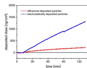
Mass loading signal on quartz crystal sensor of a QCM online measurement for diffusional and electrostatically deposited particles.
