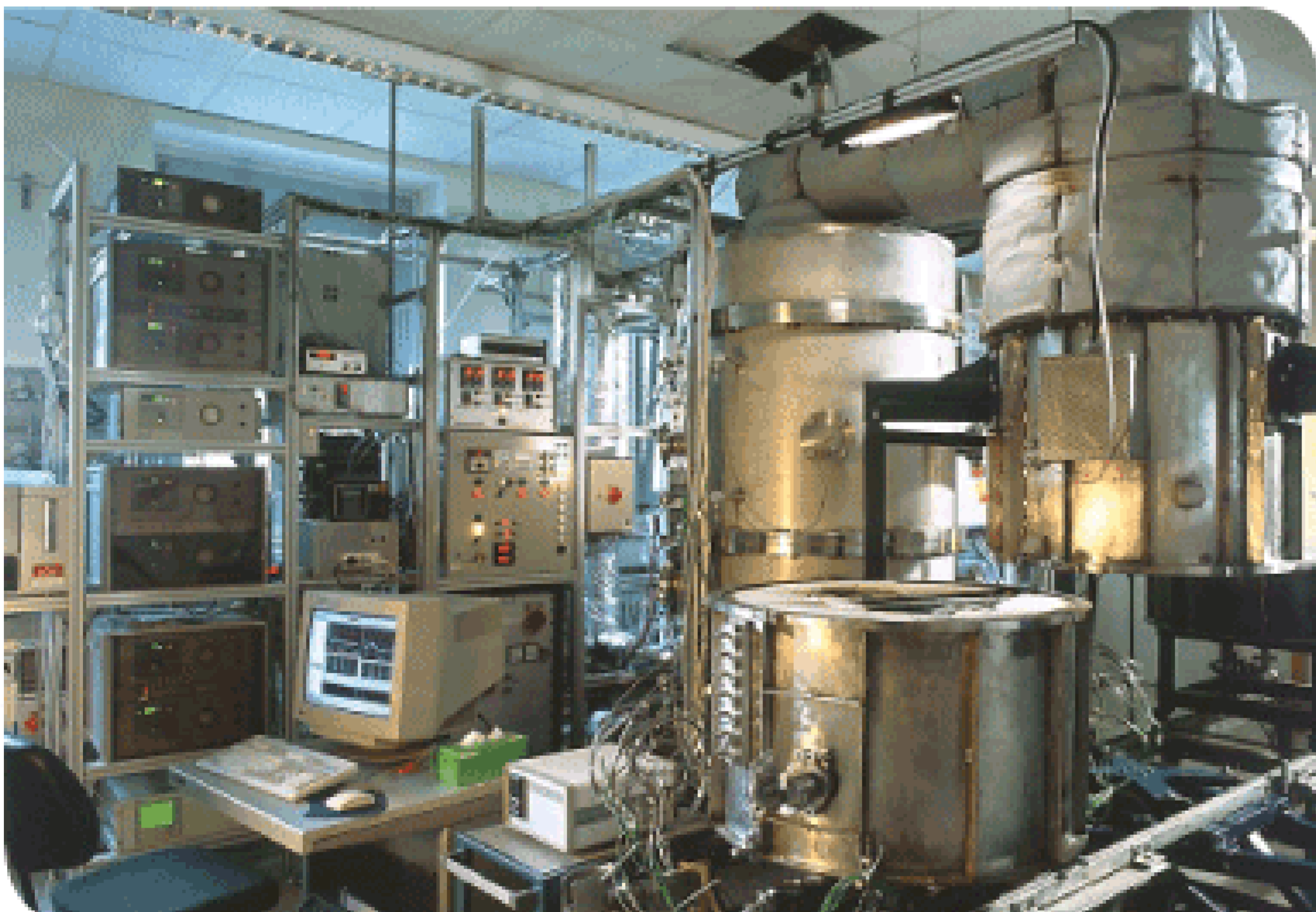
Figure 1: Fixed-bed reactor KLEAA
