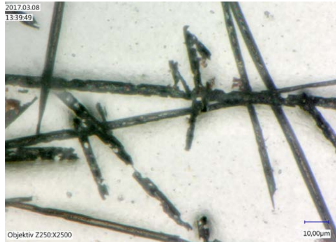
Optical microscopy image of a thermal treated CF sample (image: KIT).
