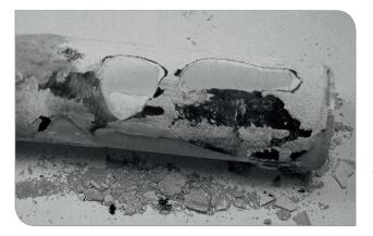
Sulfation of the fly ash and ash deposits on the boiler surface can reduce chloride concentration and, hence, formation of Cl<sub>2</sub>. The Cl/S ratio of the fly ash and ash deposits correlates with the HCl/SO<sub>2</sub> ratio of the flue gas. High  $SO_2$  concentrations reduce chloride concentration in the fly ash and ash deposits.
